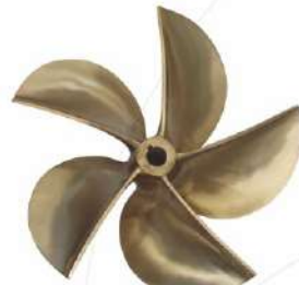
半潜桨 Surface Propellers
